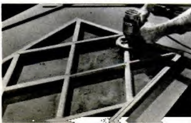
ROUTER AND SHAPED CUTTER dress up strips. Make sure that parts are numbered before disassembling
